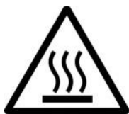
Figure 1.2 - Hot Surface Warning Label
